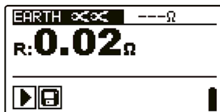
Figure 5.8: Example of contactless earthing resistance measurement result
