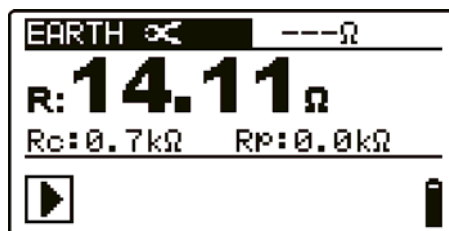
Figure 5.6: Example of selective earth resistance measurement results
